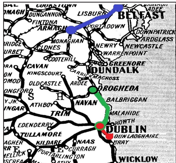
THE MAP THAT HAS BEEN ADAPTED IS FROM RAILWAY WONDERS OF THE WORLD. The first Irish railway was the Kingstown Railway, 4 ft 8½ in, shown in red. The Dublin and Drogheda was planned as 5 ft 2 in and is shown as green. The Ulster railway was built as 6 ft 2 in and is shown as blue. This map shows the full length of the Ulster Railway. Only the first 7 miles was completed in 1839.
