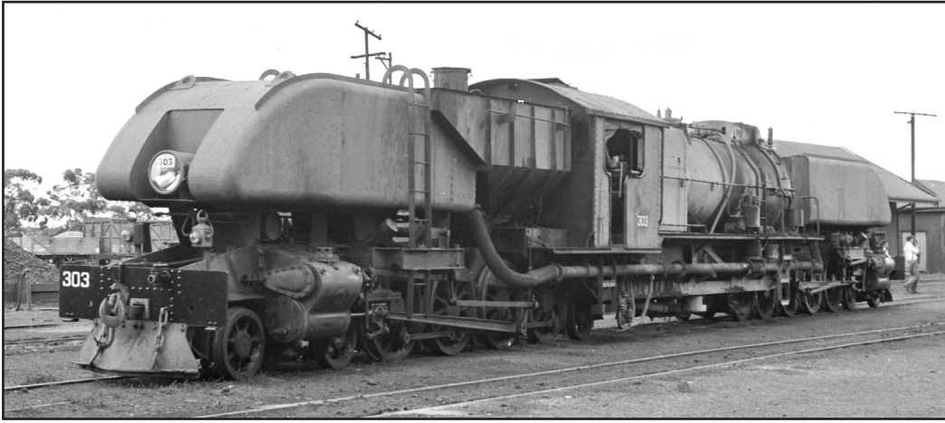
AN AUSTRALIAN STANDARD GARRATT at Peterborough. The South Australian Railways acquired six of these that became the 300 class. This is No. 303. These ASGs were not popular with engine crews. Their design had included flangeless front driving wheels with the intention that they would be able to negotiate sharp curves but it made them prone to derail. DOUG COLQUHUON, FROM THE NATIONAL RAILWAY MUSEUM.
