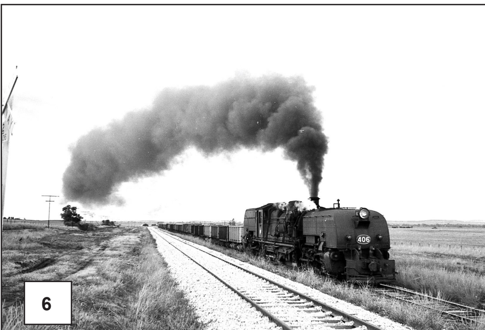
6. GARRATT No 406 OF THE SOUTH AUSTRALIAN RAILWAYS. It is doing the task for which it was purchased - the Broken Hill concentrates to the smelters at Port Pirie - but not for much longer. The new standard-gauge track is all packed down with ballast and ready for the first coast to coast freights in January 1970. There were two of these 400 class Garratts that survived and passed to rail heritage groups. 409 was the last of the class in steam and is in the National Railway Museum. No 402 went to the Zig Zag Railway. JLW.
