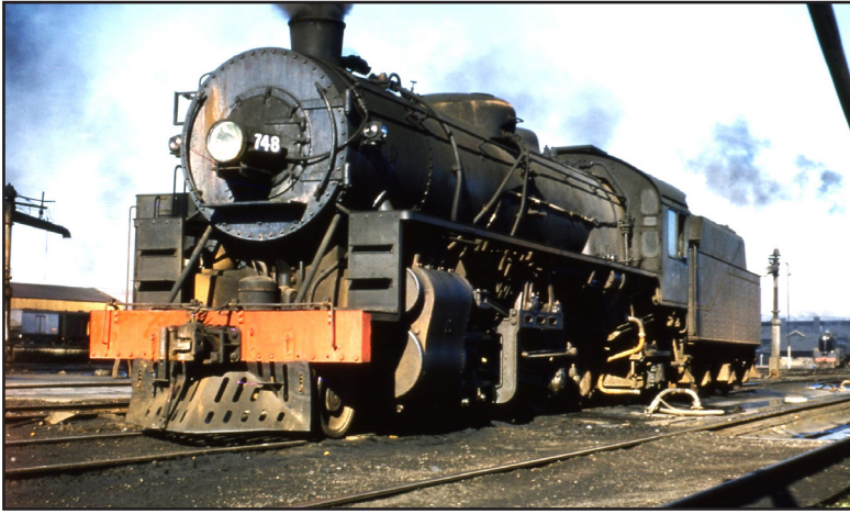
LEFT. No 748 of the South Australian Railways would have traditionally been called a 'Mikado', but in the post-war environment was a 'MacArthur'. It's design very closely followed the 700 class of the South Australian Railways GEOFF GRANT COLLECTION.
