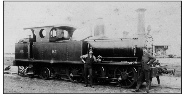
WILLIAM THOW'S K CLASS. It came in a broad-gauge version and a narrow-gauge version. K52 was the solitary narrow-gauge example. It was not a success. It worked better going bunker first, which explains the cow-catcher at the rear. NATIONAL RAILWAY MUSEUM
