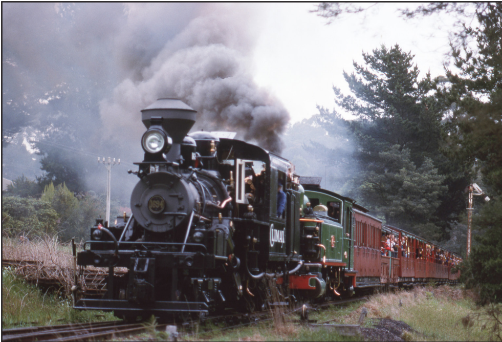
THE CLIMAX ENGINE ON THE PUFFING BILLY RAILWAY. The Climax was a locomotive with a geared drive that found favour amongst private railways servicing coal and timber operations. Credit is due to the Puffing Billy Railway for restoring this engine from a derelict state. THE COLLECTION OF THE NATIONAL RAILWAY MUSEUM.
