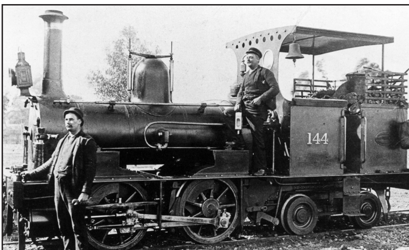
SOUTH AUSTRALIAN RAILWAYS V CLASS. These were the lightest locomotives used on the system and could just manage on the Kingston line where they replaced the horses. They also had the advantage of being small enough to be disassembled and loaded aboard the small coastal vessels that tied up at Kingston.
