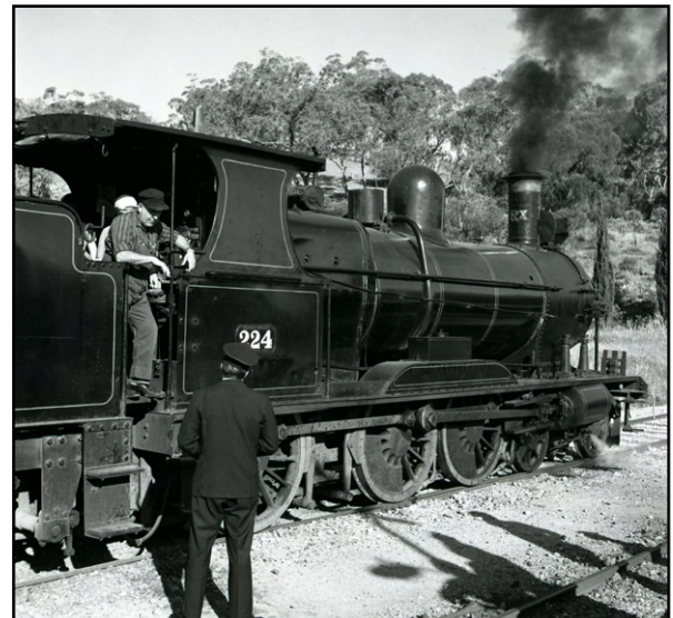
THE FLANGELESS FRONT DRIVING WHEEL of the Rx class locomotive is shown in this photograph taken at Clare. ROGER CURRIE.
