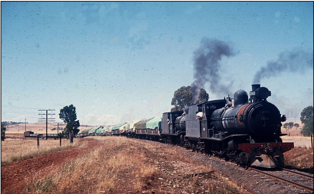
THE WILMINGTON LINE in the mid-north of South Australia was a narrow-gauge line that was built with economies as shown in this picture, in that it followed the contour of the land. This wheat train was hauled by T class engines 240 and 245. The location was Yandiah. 1 December 1965. JLW.
